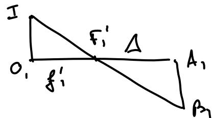
$$f'_1 = \Delta \frac{AB}{A'_1 B'_1} \quad \text{car} \quad O_1 I = AB$$
